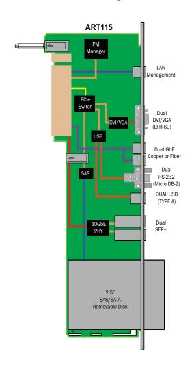
FIGURE 1. ART115 Functional Block Diagram
